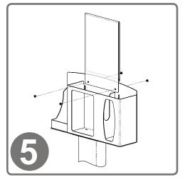
To mount the Sign Holder, place the lip of the holder over the front edge of the dispenser, lining up holes. With a lathead screwdriver, attach using (2x) barrel screws included with sign holder.
