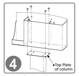
Attach the Respiratory Hygiene Station to the column using (4x) screws included with stand. Tighten.
