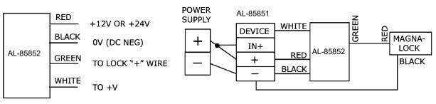
**NOTE:** Positive input voltage on the white wire must be from the same power source that the red and black wires are connected.
