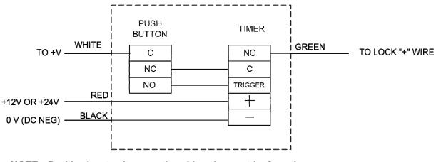
**NOTE:** Positive input voltage on the white wire must be from the same power source that the red and black wires are connected.
