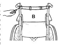
the wheelchair frame. Insert screws through grommets, into screw holes, and tighten. (See Illustration B.)
