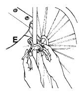
6. Place one clamp on either the left or right side of the wheelchair frame approximately three inches below the seat, (See illustration E.) Tighten screws enough so that clamp stays in place, but not so tight as to prevent clamp
