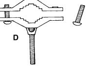
5. Remove one screw from one clamp. (See illustration D.) This clamp and screw will be used in step 7.
