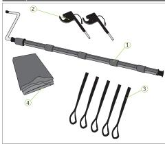
1 Transfer Bar with Handle 3 Transfer Straps (with clips) 4 Transfer Sheets 2 Chair Brackets
