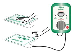
Test the system. (A) Put pressure on the sensor pad to activate the pad and the fall monitor. The fall monitor will beep two times to indicate that the sensor pad and the fall monitor are in use. The "Status" light will blink every 4 seconds while pressure remains on the pad. (B) When pressure is removed, the fall monitor will sound the alert tone. Slide the power switch to "OFF" to silence the monitor. Slide the switch to "ON" to reactivate the system.
