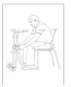
Step 2. Pull the walker as close as possible so that the skis are positioned under the seat. There are three different hand positions: pistol, medium and the recommended ball-joint grips.
