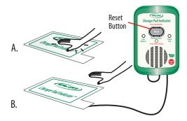
Test the system. (A) Put pressure on the sensor pad to activate the pad and the fall monitor. The fall monitor will beep two times to indicate that the sensor pad and the fall monitor are in use. The "Status" light will blink while pressure remains on the pad. (B) When pressure is removed, the fall monitor will sound the alert tone. Press the Reset button to silence the alert.
