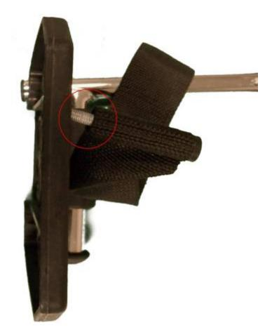
8. Tighten the screw with an Allen wrench.
