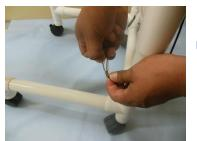
Delta PLACE THE METAL FERRELS ON THE EXPOSED PART OF THE WIRE FIRST THEN THE CLEAR PLASTIC.
