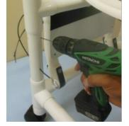
DRILL A HOLE ON THE LEFT TOP CORNER OF THE VERTICAL PIPE (LEFT WHEN SEATING) 1" FROM THE TEE FITTING USE A 1/8 BIT.
