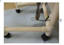
PUSH THE EXPOSED WIRE THROUGH THE FERREL BEFORE CRIMPING.
