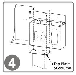
Attach the Respiratory Hygiene Station to the column using (4x) screws included with stand. Tighten.
