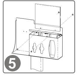
To mount the Sign Holder, align the mounting holes of the holder with the holes on the top front of the dispenser. Attach using (2x) barrel screws included with sign holder.
