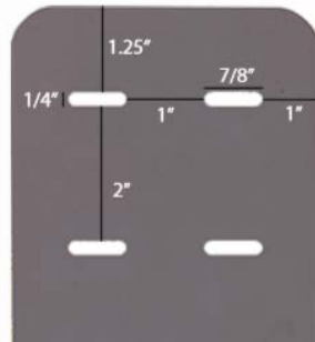
Backplate A Mounting Dimensions
