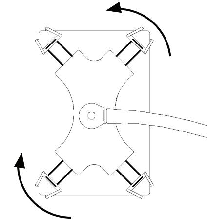
The head of the Tab Grabber can be rotated 360 ° on both axes for optimal positioning.
