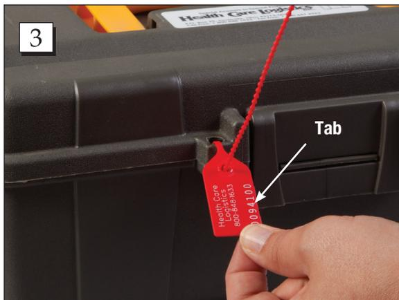
**Step 3.** Utilize the "TUG" test by grasping the tab of the seal, gently tug on it to determine closure. If you are able to loosen the seal, IT IS NOT FULLY LOCKED. Remove the seal and replace with a new one.
