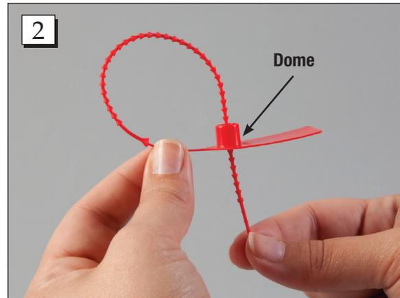
**Step 2.** Pull the stem through the locking dome on the side marked "Enter". Pull it as tight as possible around the item being sealed. This will ensure that the seal stem cannot be broken and reinserted into the locking mechanism.
