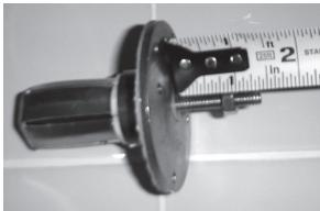
9. Measure out the thickness of the wall on the **WingIt™** and back off the nut accordingly. For example, picture #8 shows a wall thickness of 3/4" (19mm). In this example you would back off the nut 3/4" (19mm) on the **WingIt™**. This will allow adequate clearance.
