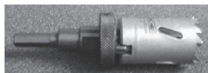
4. A Sandvik Carbide tipped Hole Saw [Available through WingIt™ – with 3/8" (9mm) arbor], will drill a 1-1/4" (30mm) hole at slow speeds in a matter of seconds and remain sharp for 30–80 holes, depending on the tile.
