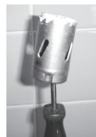
5. After the initial 1-1/4" (30mm) hole is made through the tile, stop, and eject the tile from the drill bit.
