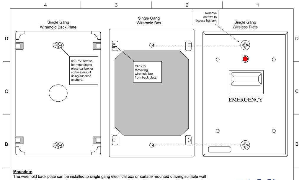
The wiremold back plate can be installed to single gang electrical box or surface mounted utilizing suitable wall anchors for the type of wall. Alternative mounting may be accomplished utilizing double-faced foam tape or hook and loop fastener.
