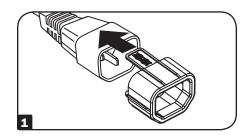
Securely connect the C14 or C20 equipment plug to a C13 or C19 power source.
