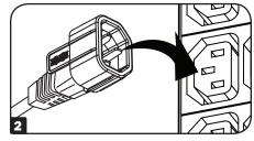
To disconnect the equipment plug from the power source, grip the plug **A** and plug lock tabs **B** simultaneously and then remove them from the power source.
